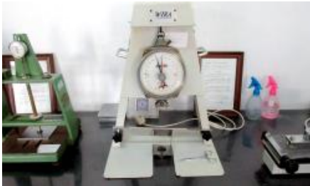
Tuft Pullout Tester
