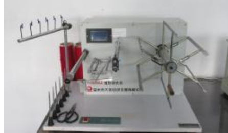
Yarn Length Measuring Machine
