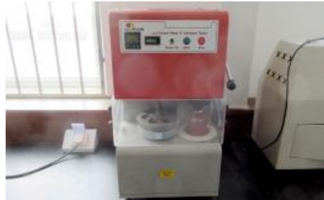
Carpet Wear and Abrasion Tester
